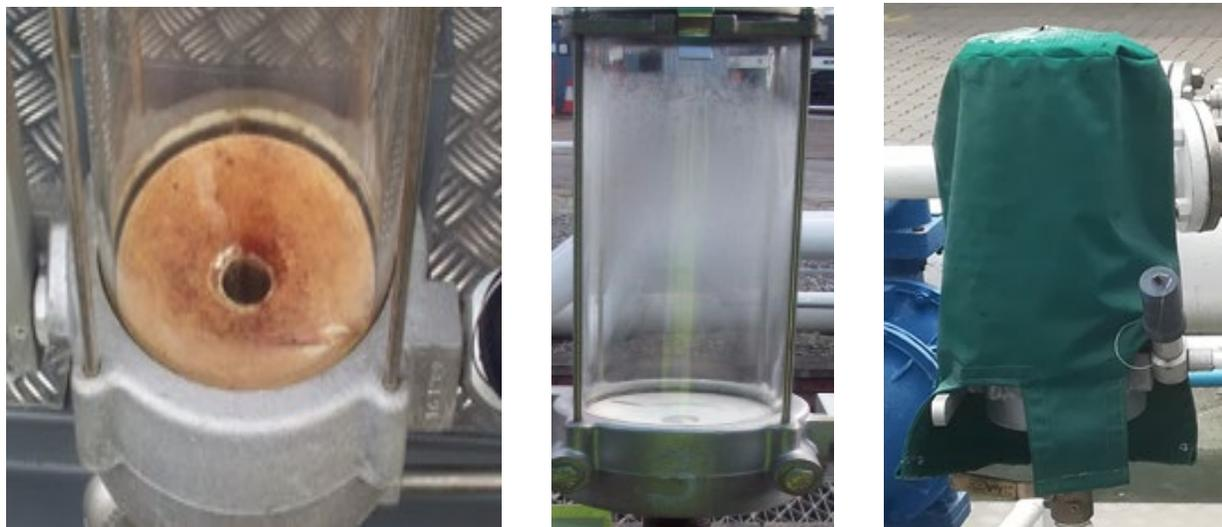
'Visijars' should also be routinely inspected to confirm general condition and that there are no leaks (e.g. cracks in the glass or failed seals between the glass and the base). Any leaks observed from closed-circuit samplers are not acceptable and the equipment should not be used until the defect has been corrected (e.g. replacement parts have been fitted).
