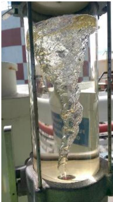
Therefore, no accessories that disrupt or prevent the formation of a vortex shall be installed in a 'Visijar' during sampling or Visual Appearance Checks.
